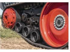
Our patented Mobil-Trac System (MTS) provides an operator with better traction, and with reduced compaction, thanks to its long footprint and pivoting midwheel design. Paired with our Smart Ride and cab suspension system, it provides exceptional ride quality down the road or through the field.
