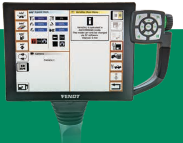
Monitor and adjust all tractor functions, including the transmission, hydraulic system, 3-point hitch, headland management system, service and diagnostics.
